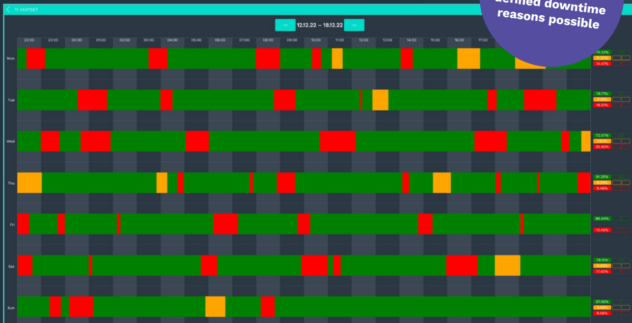
Exemplary display of a milling machine with downtimes and productive times including piece counting
